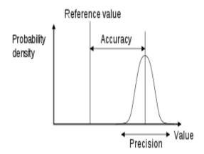
Accuracy indicates proximity of measurement results to the true value, precision to the repeatability or reproducibility of the measurement
