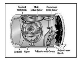
The heading indicator (or directional gyro) is fundamentally a mechanical instrument designed to facilitate the use of the magnetic compass.
