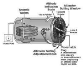
The altimeter shows the aircraft's height above sea-level by measuring the difference between the pressure in a stack of aneroid capsules inside the altimeter and the atmospheric pressure obtained through the static system.
