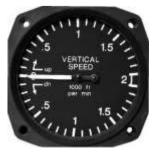
The VSI (also sometimes called a variometer) Sense changing air pressure, and displays that information to the pilot as a rate of climb or descent in feet per minute, meters per second or knots. only one needle, a typical RMI has two, coupled to different ADF receivers, allowing for position fixing using one instrument.
