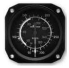
The airspeed indicator shows the aircraft's speed (usually in knots) relative to the surrounding air. It works by measuring the ram-air pressure in the aircraft's Pitot tube.
