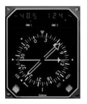
An RMI is generally coupled to an automatic direction finder (ADF), which provides bearing for a tuned Non-directional beacon (NDB). While simple ADF displays may have
