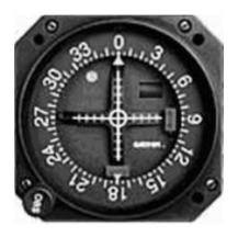
The CDI is an avionics instrument used in aircraft navigation to determine an aircraft's lateral position in relation to a track, which can be provided by a VOR or a System. This instrument can also be integrated with the heading indicator in a horizontal situation indicator.
