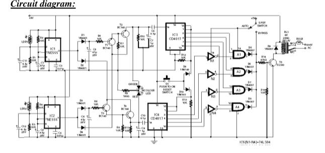
The next stage comprises two logic ICs which can combine the outputs of the two counters and determine if there is any person still left in the room or not.
