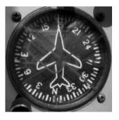
The heading indicator (also known as the directional gyro, or DG; called sometimes also the gyrocompass, though usually not in aviation applications) displays the aircraft's heading with respect to geographical north. Principle of operation is a spinning gyroscope, and is therefore subject to drift errors (called precession) which must be periodically corrected by calibrating
